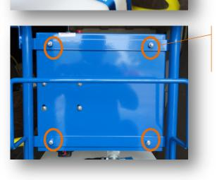
Remove Locking screw - When closing box Only hand tighten
